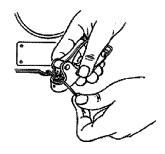
Pass wire through item to be sealed. Insert wire end or ends into Alucast seal. Pull wire tight to decrease loop size.
