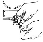
2. Fit seal into jaws of sealing tool and firmly compress handles.
